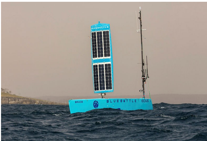
Figure 6.1: Ocius's BlueBottle unmanned surface vessel
